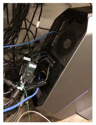
Back of the PC with 18 DVI cables connected to 18 mini-displayport adapters.
