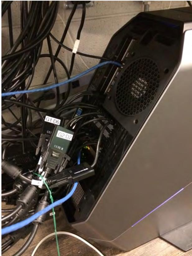
Back of the PC with 18 DVI cables connected to 18 mini-displayport adapters.
