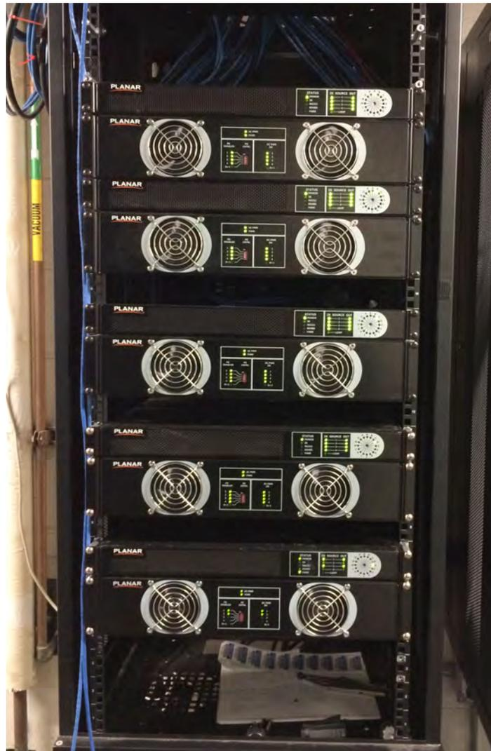
Planar Quad power and controller: 5 pairs of boxes (old Gen1 model, controller + power): 1 rack is enough for our 18 screens.
