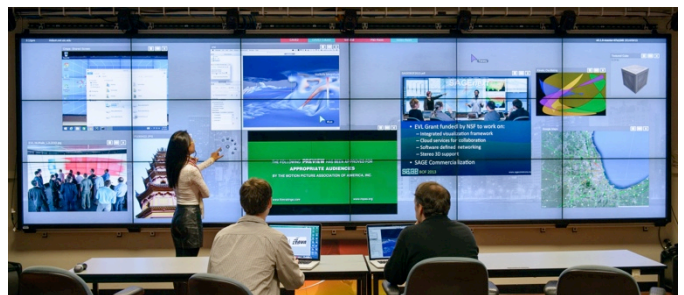
Fig. 1. A typical SAGE2 session, depicting multiple applications windowed on a SRSD. This figure illustrates the wide array of content supported by SAGE2, including images, videos, PDFs, 2D and 3D custom applications, and an off-the-shelf application from a remote source.
